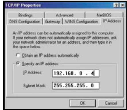
Photo 3 —Configuring a NIC card in a desktop PC to talk TCP/IP is completely painless under Win95/98. Simply edit the TCP/IP properties IP address tab and assign your IP address and sub-network mask.
