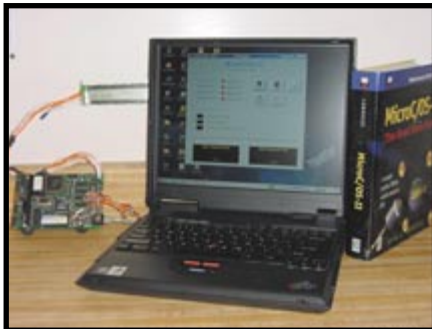
Photo 5 —Commands from the GUI are sent down the Ethernet pipe via UDP datagrams. A/D readings, digital input status, and kernel statistics are sent from the TS-2800 to the PC via UDP datagrams Ethernet-style and embedded.
