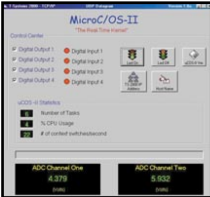
Photo 4 —The GUI resides on the host computer. All of the real-time work is handled on the TS-2800, which is powered by the MicroC/OS-II application.
